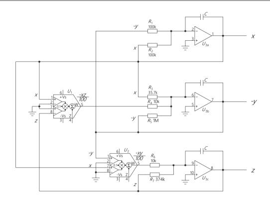
$U_1U_2$  = AD633JR SO-8 CAUTION: DIP and SO packages have different pinouts  $U_3$  = LM324N  $R_1R_7$  = Hand selected for accuracy C = 0.1 $\mu$ F  $C_d$  = 0.1 $\mu$ F
